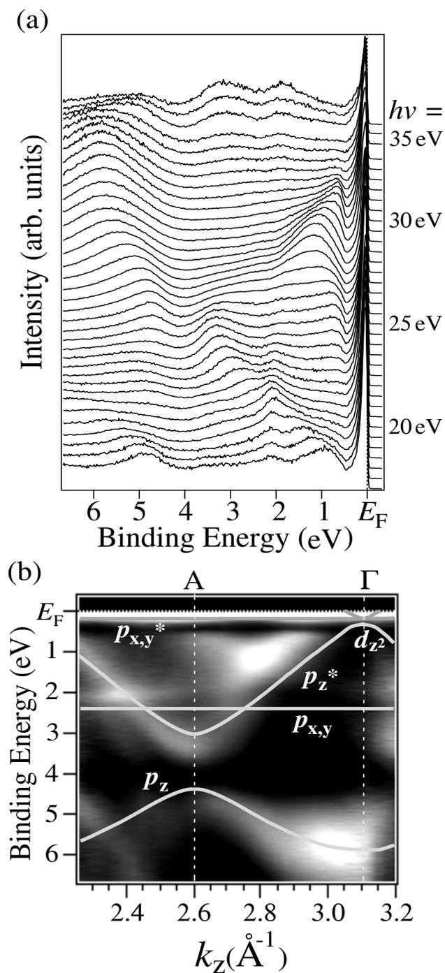
Fig. 1. (a) Normal-emission valence-band ARPES spectra of 1T-VSe<sub>2</sub> measured at 30 K. Photon energy ( $h\nu$ ) is denoted on spectra. (b) Comparison of the experimental valence-band structure (gray scale) with the LAPW band calculation (solid lines)<sup>11)</sup> along the  $\Gamma A$  direction. Bright areas correspond to bands.
