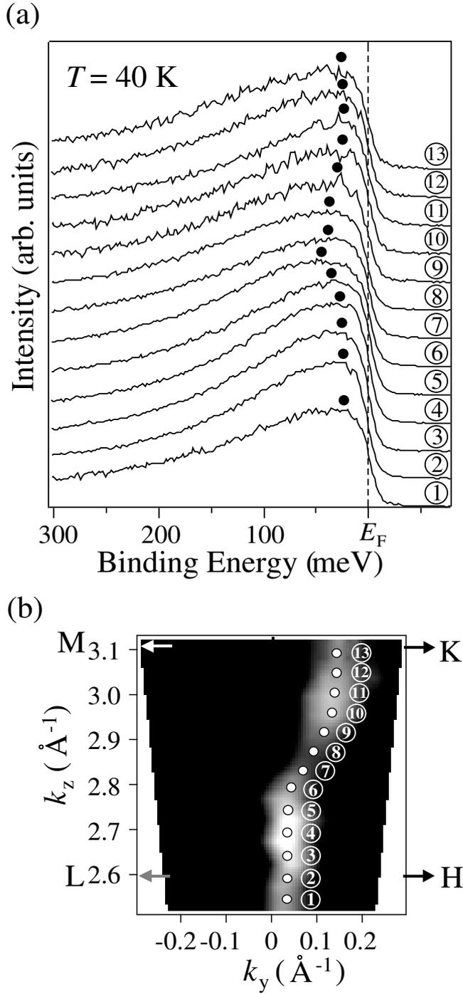
Fig. 3. (a) ARPES spectra in the vicinity of  $E_F$  at 40 K for 1T-VSe<sub>2</sub>, measured at various positions on the FS denoted by number (1 to 13) in (b). The peak position in spectra determined by fitting with Gaussian around the peak top is indicated by filled circles.
