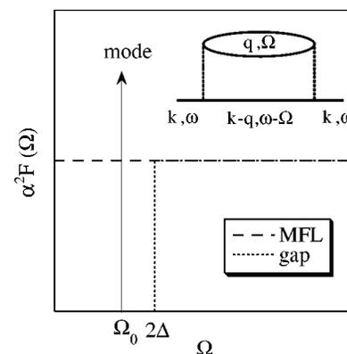
FIG. 1.  $\alpha^2F$  for three models, MFL (dashed line), gapped MFL (dotted line), and gapped MFL plus mode (dotted line plus  $\delta$  function). Inset: Feynman diagram for the lowest-order contribution to  $\Sigma$  from electron-electron scattering.
