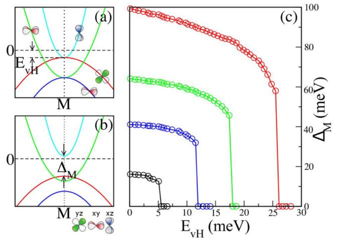
FIG. 6. (a) Schematics of the electronic structure near  $M$  showing the location of the vHS ( $E_{\text{vH}}$ ) before (a) and the degeneracy splitting energy  $\Delta_M$  after (b) the nematic transition. (c)  $\Delta_M$  as a function of  $E_{\text{vH}}$  at fixed  $V_0/V = 1.8, 1.7, 1.6, 1.4$  from the top line to the bottom line.
