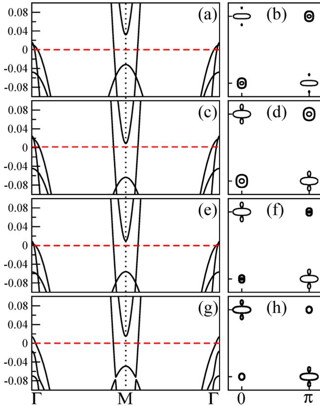
FIG. 5. Band dispersion in units of eV (left panel) and FS (right panel) in a  $d$ -wave nematic state. (a) and (b)  $V = 0.763$  eV,  $E_{vH} = 0$ , and  $V_0 = 1.3$  eV. (c) and (d)  $V = 0.73$  eV,  $E_{vH} = 25$  meV, and  $V_0 = 1.34$  eV. (e) and (f)  $V = 0.75$  eV and  $V_0 = 1.325$  eV at 1% electron doping. (g) and (h) With SOC  $\lambda_{\text{soc}} = 28$  meV,  $V = 0.763$  eV,  $V_0 = 1.32$  eV at 1% electron doping.
