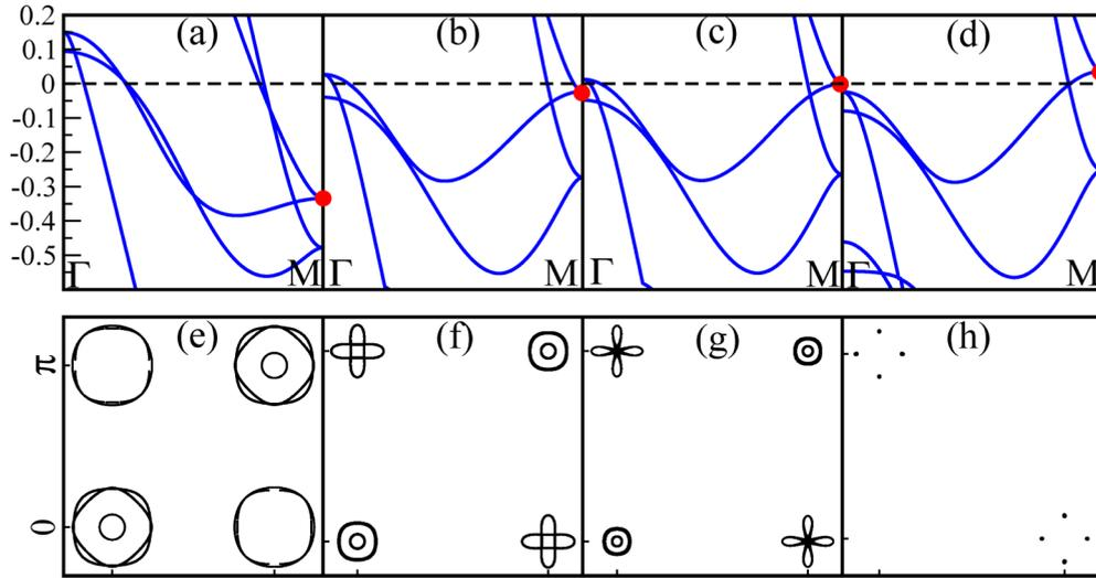
FIG. 3. Renormalized band structure (a)–(d) in unit of eV and corresponding FS (e)–(h) at  $V = 0$  (a), 0.73 eV (b), 0.763 eV (c), and 0.85 eV (d). Red dots indicate vHS at  $d_{xz/yz}$  degeneracy point at  $M$ . FSs in (e) are 87.5% of their actual sizes.
