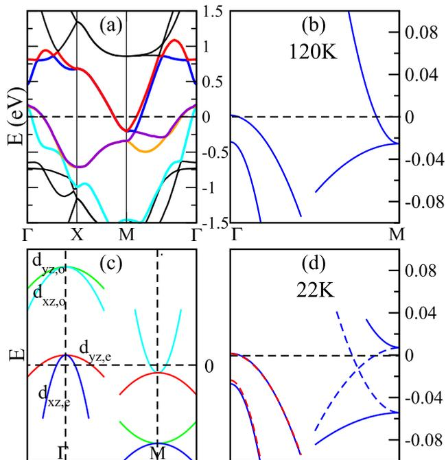
FIG. 1. (a) LDA band structure of FeSe. (b) Band dispersions observed by ARPES in the symmetric phase at 120 K. (c) Band degeneracy at high-symmetry points ( $\Gamma, M$ ) among  $d_{xz,e}$  (blue),  $d_{yz,e}$  (red),  $d_{xz,o}$  (cyan), and  $d_{yz,o}$  (green). (d) ARPES results in the nematic state at 22 K. Red dashed lines near  $\Gamma$  are data taken at 120 K, showing  $\Delta_{\Gamma}$  is nearly  $T$ -independent. Solid and dashed blue lines near  $M$  correspond to the two domains.
