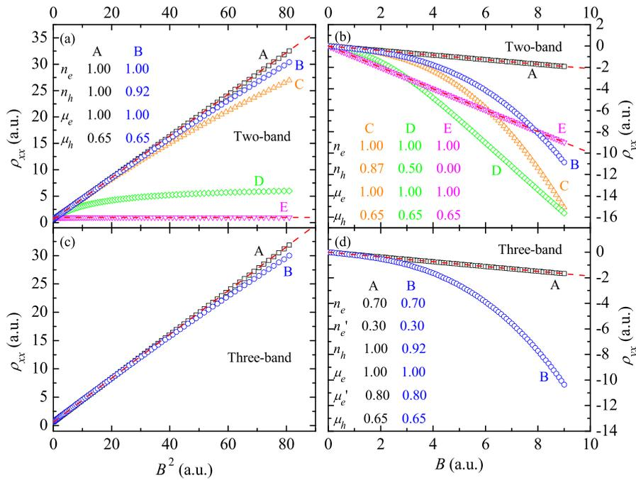
FIG. 3. Numerical simulations of  $\rho_{xx}(B)$  (left panels) and  $\rho_{yx}(B)$  (right panels). The parameters are listed in panels (a), (b), and (d). The red dashed lines are the linear guides to the eyes. (a) and (b) are calculated with a two-band model. (c) and (d) are calculated with a three-band model.
